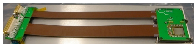
Figure 12. Packaged BTBV12M detector from Teledyne.
